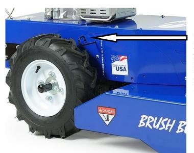
Free wheeling lever, push in for unit to move under power. Pull out to push unit manually with engine off.
