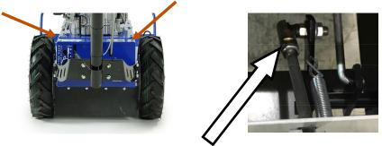
• The forward and reverse linkage is threaded into the coupling, thread the lower fitting all the way in and tighten the jam nut on the rod to the fitting. The upper fitting should be close to flush with the end. Insert fitting in hand lever linkage and insert hairpin. When set up correct the unit will have equal forward and reverse movement.
