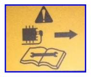
Disconnect spark plug and read manual before servicing the equipment
